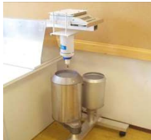
Rain gauge calibration unit
