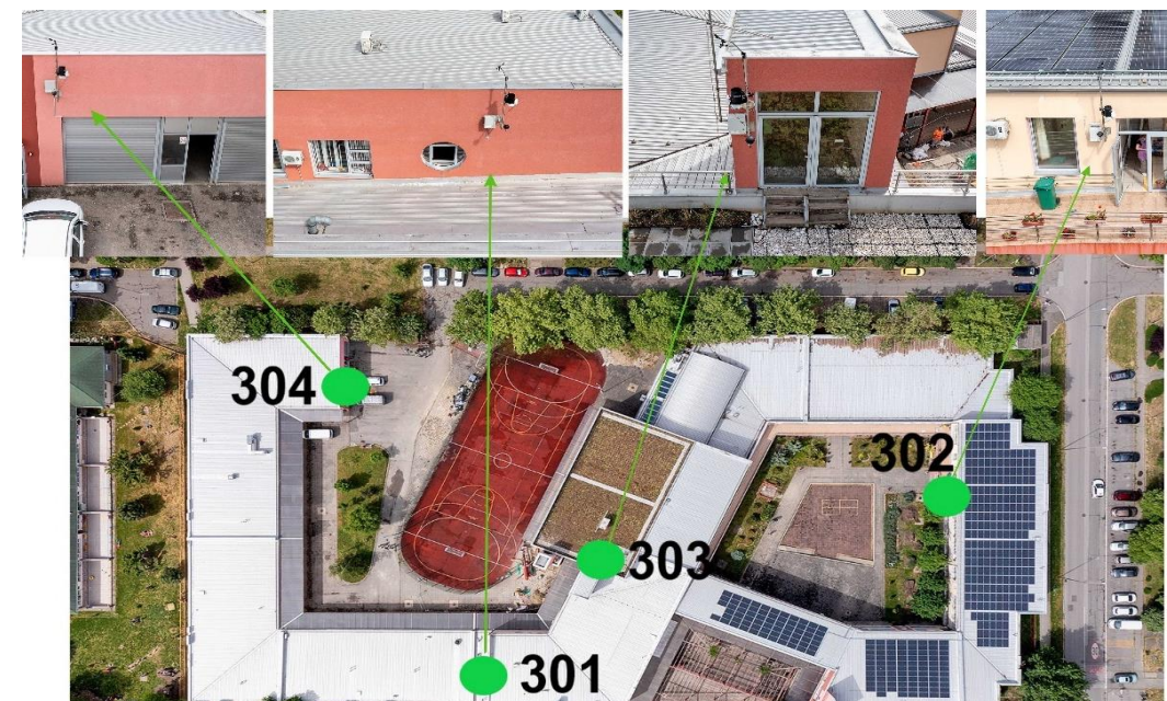
Fig. 2. Green roof and installed weather stations in Novi Sad, Serbia (Savić et al., 2023)
